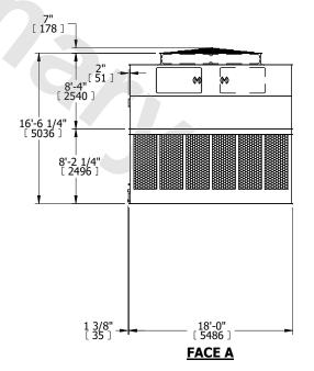
SHIPPING WEIGHT 22160 lbs+ [10055] kg+ OPERATING WEIGHT 40700 lbs+ [18465] kg+ HEAVIEST SECTION WEIGHT 6700 lbs+ [3040] kg+ NO. OF SHIPPING SECTIONS 4 DRAWN BY: KDS
