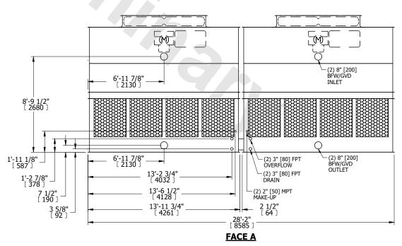
SHIPPING WEIGHT 11700 lbs+ [5310] kg+ OPERATING WEIGHT 20720 lbs+ [9400] kg+ HEAVIEST SECTION WEIGHT 3710 lbs+ [1685] kg+ NO. OF SHIPPING SECTIONS 4 DRAWN BY: JLG
