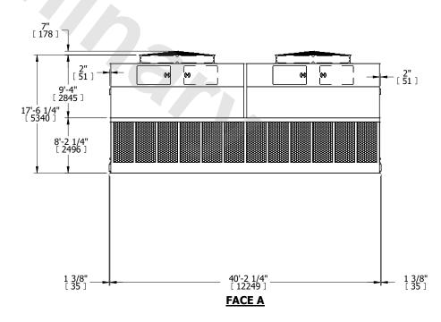
SHIPPING WEIGHT 51440 lbs+ [23335] kg+ OPERATING WEIGHT 92640 lbs+ [42025] kg+ HEAVIEST SECTION WEIGHT 9000 lbs+ [4085] kg+ NO. OF SHIPPING SECTIONS 6 DRAWN BY: BLL
