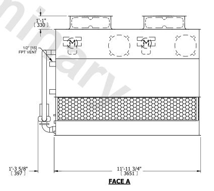
DRAWN BY: CAF NO. OF SHIPPING SECTIONS **SHIPPING** OPERATING HEAVIEST SECTION 4890 lbs+ [2220] kg+ 5710 lbs+ [2595] kg+ 8870 lbs+ [4025] kg+ WEIGHT WEIGHT WEIGHT
