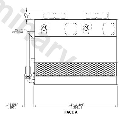
DRAWN BY: NO. OF SHIPPING SECTIONS **SHIPPING** OPERATING HEAVIEST SECTION 6490 lbs+ [2945] kg+ 9910 lbs+ [4500] kg+ 5670 lbs+ [2575] kg+ WEIGHT WEIGHT WEIGHT
