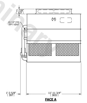
DRAWN BY: SLR NO. OF SHIPPING SECTIONS **SHIPPING OPERATING** HEAVIEST SECTION 8360 lbs+ [3795] kg+ 10160 lbs+ [4610] kg+ 15600 lbs+ [7080] kg+ WEIGHT WEIGHT WEIGHT
