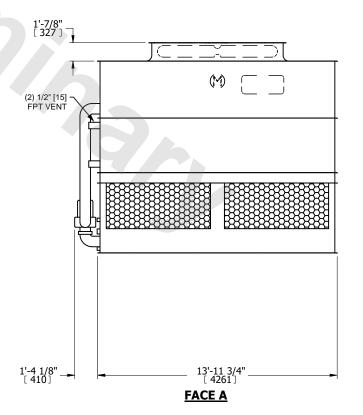
DRAWN BY: SLR NO. OF SHIPPING SECTIONS **SHIPPING** OPERATING HEAVIEST SECTION 13330 lbs+ [6050] kg+ 20300 lbs+ [9210] kg+ 11320 lbs+ [5135] kg+ WEIGHT WEIGHT WEIGHT
