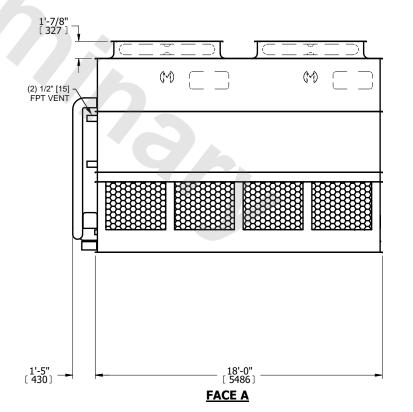
SHIPPING WEIGHT 20320 lbs+ [9220] kg+ OPERATING WEIGHT 30180 lbs+ [13690] kg+ HEAVIEST SECTION WEIGHT 17530 lbs+ [7955] kg+ NO. OF SHIPPING SECTIONS 2 DRAWN BY: SLR
