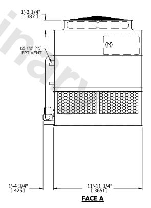
DRAWN BY: SLR NO. OF SHIPPING SECTIONS **SHIPPING** OPERATING HEAVIEST SECTION 14150 lbs+ [6420] kg+ 16860 lbs+ [7650] kg+ 26300 lbs+ [11930] kg+ WEIGHT WEIGHT WEIGHT
