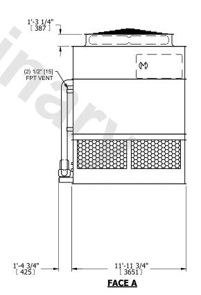
**SHIPPING** OPERATING HEAVIEST SECTION 24020 lbs+ [10900] kg+ 21310 lbs+ [9670] kg+ 35900 lbs+ [16285] kg+ WEIGHT WEIGHT WEIGHT
