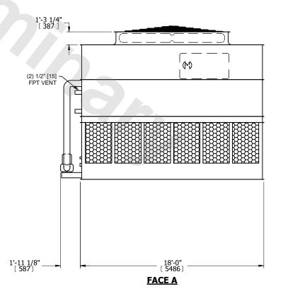
SHIPPING WEIGHT 20290 lbs+ [9205] kg+ OPERATING WEIGHT 33230 lbs+ [15075] kg+ HEAVIEST SECTION WEIGHT 16370 lbs+ [7430] kg+ NO. OF SHIPPING SECTIONS 2 DRAWN BY: SLR
