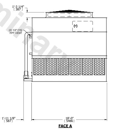
SHIPPING WEIGHT 30460 lbs+ [13820] kg+ OPERATING WEIGHT 47080 lbs+ [21360] kg+ HEAVIEST SECTION WEIGHT 26540 lbs+ [12040] kg+ NO. OF SHIPPING SECTIONS 2 DRAWN BY: SLR
