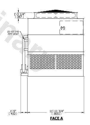
DRAWN BY: SLR NO. OF SHIPPING SECTIONS **SHIPPING** OPERATING HEAVIEST SECTION 12390 lbs+ [5625] kg+ 19900 lbs+ [9030] kg+ 9840 lbs+ [4465] kg+ WEIGHT WEIGHT WEIGHT
