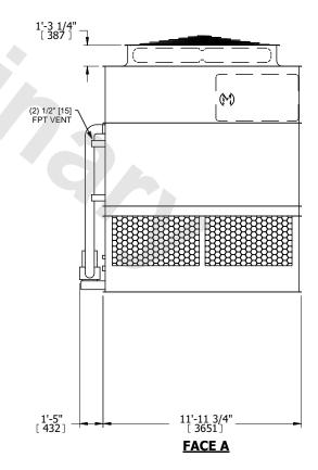
SHIPPING WEIGHT 16050 lbs+ [7285] kg+ OPERATING WEIGHT 24880 lbs+ [11290] kg+ HEAVIEST SECTION WEIGHT 13500 lbs+ [6125] kg+ NO. OF SHIPPING SECTIONS 2 DRAWN BY: SLR
