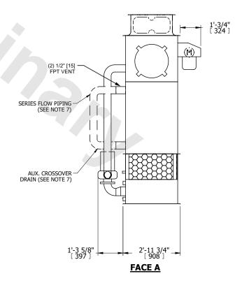
DRAWN BY: NO. OF SHIPPING SECTIONS **SHIPPING OPERATING** HEAVIEST SECTION 1600 lbs+ [730] kg+ 2260 lbs+ [1030] kg+ 1320 lbs+ [600] kg+ WEIGHT WEIGHT WEIGHT
