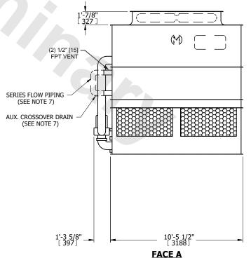
DRAWN BY: JLG NO. OF SHIPPING SECTIONS HEAVIEST SECTION 13930 lbs+ [6320] kg+ 7610 lbs+ [3455] kg+ WEIGHT
