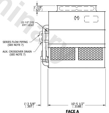
DRAWN BY: JLG NO. OF SHIPPING SECTIONS **SHIPPING** OPERATING HEAVIEST SECTION 7790 lbs+ [3535] kg+ 9430 lbs+ [4280] kg+ 14110 lbs+ [6405] kg+ WEIGHT WEIGHT WEIGHT
