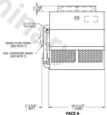
DRAWN BY: JLG NO. OF SHIPPING SECTIONS **SHIPPING** OPERATING HEAVIEST SECTION 10720 lbs+ [4865] kg+ 15890 lbs+ [7210] kg+ 9080 lbs+ [4120] kg+ WEIGHT WEIGHT WEIGHT
