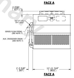
DRAWN BY: JLG NO. OF SHIPPING SECTIONS **SHIPPING** OPERATING HEAVIEST SECTION 19880 lbs+ [9020] kg+ 30760 lbs+ [13955] kg+ 8140 lbs+ [3695] kg+ WEIGHT WEIGHT WEIGHT
