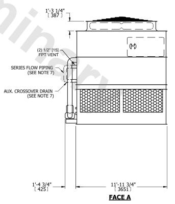
DRAWN BY: TLM NO. OF SHIPPING SECTIONS **SHIPPING** OPERATING HEAVIEST SECTION 14390 lbs+ [6530] kg+ 23010 lbs+ [10440] kg+ 11680 lbs+ [5300] kg+ WEIGHT WEIGHT WEIGHT
