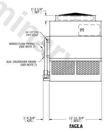
DRAWN BY: JLG NO. OF SHIPPING SECTIONS **SHIPPING** OPERATING HEAVIEST SECTION 18830 lbs+ [8545] kg+ 29080 lbs+ [13195] kg+ 16120 lbs+ [7315] kg+ WEIGHT WEIGHT WEIGHT
