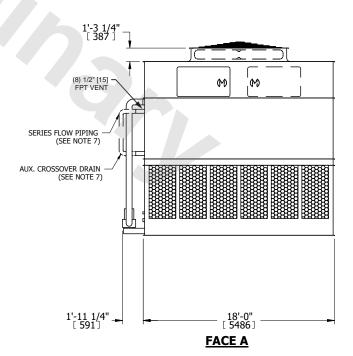
SHIPPING 59120 lbs+ [26820] kg+ OPERATING WEIGHT 89640 lbs+ [40665] kg+ HEAVIEST SECTION WEIGHT 25890 lbs+ [11745] kg+
