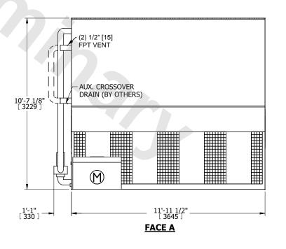
DRAWN BY: NO. OF SHIPPING SECTIONS **SHIPPING** OPERATING HEAVIEST SECTION 8680 lbs+ [3940] kg+ 12820 lbs+ [5820] kg+ 5930 lbs+ [2690] kg+ WEIGHT WEIGHT WEIGHT
