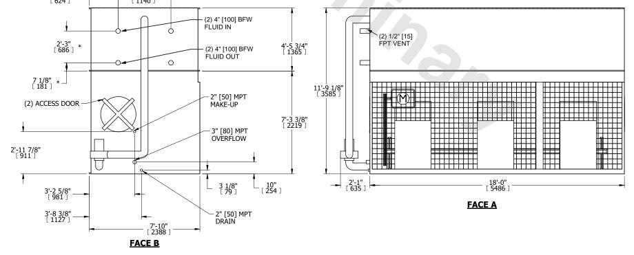
**SHIPPING** OPERATING HEAVIEST SECTION 16300 lbs+ [7395] kg+ 24680 lbs+ [11195] kg+ 10890 lbs+ [4940] kg+ WEIGHT WEIGHT WEIGHT
