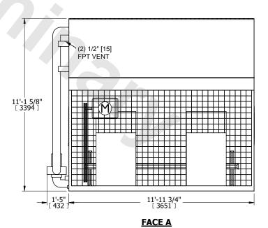
SHIPPING WEIGHT 11400 lbs+ [5175] kg+ OPERATING WEIGHT 16440 lbs+ [7460] kg+ HEAVIEST SECTION WEIGHT 7610 lbs+ [3455] kg+ NO. OF SHIPPING SECTIONS
