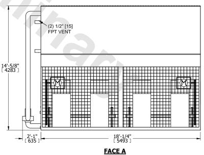
SHIPPING WEIGHT 29670 | lbs+ [13460] kg+ | OPERATING WEIGHT 41410 | lbs+ [18785] kg+ | HEAVIEST SECTION WEIGHT 22480 | lbs+ [10200] kg+ | NO. OF SHIPPING SECTIONS 2 | DRAWN BY: TLS
