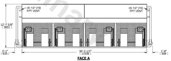
**SHIPPING** OPERATING HEAVIEST SECTION NO. OF SHIPPING SECTIONS 14820 lbs+ [6725] kg+ 43960 lbs+ [19940] kg+ 63470 lbs+ [28790] kg+ WEIGHT WEIGHT WEIGHT
