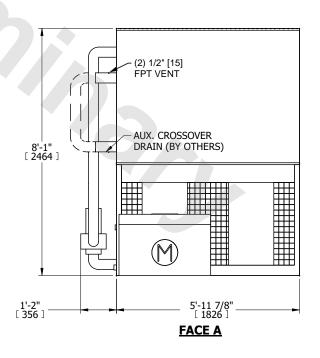
SHIPPING WEIGHT 3590 lbs+ [1630] kg+ OPERATING WEIGHT 4750 lbs+ [2155] kg+ HEAVIEST SECTION WEIGHT 2460 lbs+ [1120] kg+ NO. OF SHIPPING SECTIONS 2 DRAWN BY: TLS
