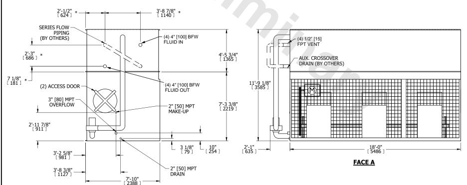
DRAWN BY: NO. OF SHIPPING SECTIONS **SHIPPING** OPERATING HEAVIEST SECTION 19720 lbs+ [8945] kg+ 28100 lbs+ [12750] kg+ 14310 lbs+ [6495] kg+ WEIGHT WEIGHT WEIGHT
