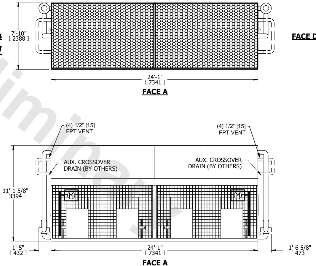
SHIPPING WEIGHT 22280 lbs+ [10110] kg+ OPERATING WEIGHT 32430 lbs+ [14715] kg+ HEAVIEST SECTION WEIGHT 7610 lbs+ [3455] kg+ NO. OF SHIPPING SECTIONS 3 DRAWN BY: TLS
