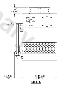
DRAWN BY: NO. OF SHIPPING SECTIONS **SHIPPING OPERATING** HEAVIEST SECTION 2710 lbs+ [1230] kg+ 3220 lbs+ [1465] kg+ 4740 lbs+ [2155] kg+ WEIGHT WEIGHT WEIGHT
