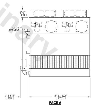
**SHIPPING** OPERATING HEAVIEST SECTION 4790 lbs+ [2175] kg+ 5460 lbs+ [2480] kg+ 7850 lbs+ [3565] kg+ WEIGHT WEIGHT WEIGHT
