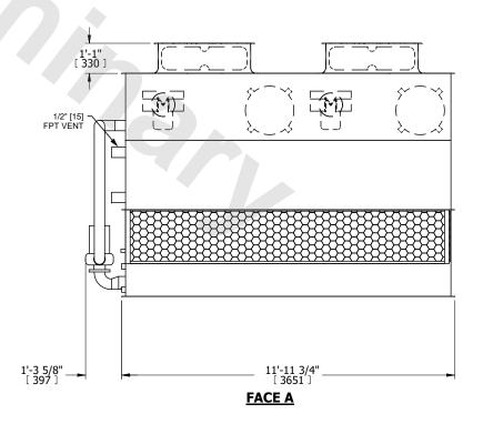
DRAWN BY: **SHIPPING** OPERATING HEAVIEST SECTION NO. OF SHIPPING SECTIONS 5760 lbs+ [2615] kg+ 8660 lbs+ [3930] kg+ 4940 lbs+ [2245] kg+ WEIGHT WEIGHT WEIGHT
