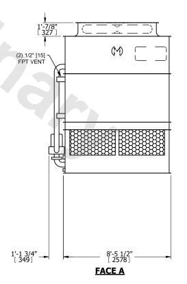
DRAWN BY: SLR NO. OF SHIPPING SECTIONS **SHIPPING** OPERATING HEAVIEST SECTION 10910 lbs+ [4950] kg+ 15090 lbs+ [6845] kg+ 9610 lbs+ [4360] kg+ WEIGHT WEIGHT WEIGHT
