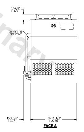
DRAWN BY: SLR NO. OF SHIPPING SECTIONS **SHIPPING OPERATING** HEAVIEST SECTION 14610 lbs+ [6630] kg+ 13170 lbs+ [5975] kg+ 19850 lbs+ [9005] kg+ WEIGHT WEIGHT WEIGHT
