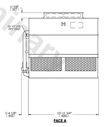
DRAWN BY: SLR NO. OF SHIPPING SECTIONS **SHIPPING OPERATING** HEAVIEST SECTION 18700 lbs+ [8485] kg+ 26320 lbs+ [11940] kg+ 16620 lbs+ [7540] kg+ WEIGHT WEIGHT WEIGHT
