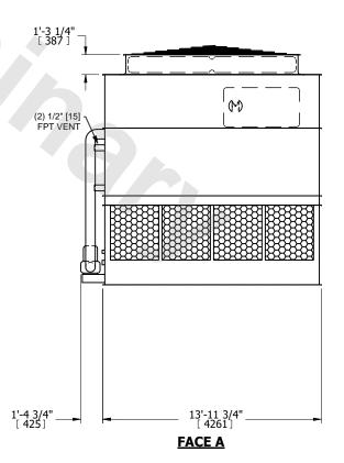
DRAWN BY: SLR NO. OF SHIPPING SECTIONS **SHIPPING** OPERATING HEAVIEST SECTION 20050 lbs+ [9095] kg+ 23110 lbs+ [10485] kg+ 34140 lbs+ [15490] kg+ WEIGHT WEIGHT WEIGHT
