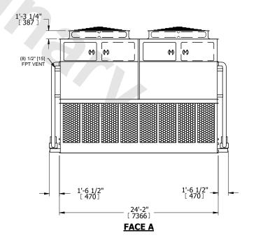
DRAWN BY: NO. OF SHIPPING SECTIONS **SHIPPING OPERATING** HEAVIEST SECTION 23970 lbs+ [10875] kg+ 107060 lbs+ [48565] kg+ 151320 lbs+ [68640] kg+ WEIGHT WEIGHT WEIGHT
