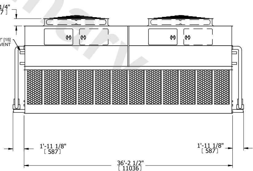
SHIPPING WEIGHT 97680 lbs+ [44310] kg+ OPERATING WEIGHT 150080 lbs+ [68080] kg+ HEAVIEST SECTION WEIGHT 20470 lbs+ [9290] kg+ NO. OF SHIPPING SECTIONS 6 DRAWN BY: SLR
