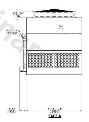
DRAWN BY: SLR NO. OF SHIPPING SECTIONS **SHIPPING** OPERATING HEAVIEST SECTION 12260 lbs+ [5565] kg+ 14810 lbs+ [6720] kg+ 22320 lbs+ [10125] kg+ WEIGHT WEIGHT WEIGHT
