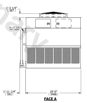
SHIPPING WEIGHT 65040 lbs+ [29505] kg+ OPERATING WEIGHT 93540 lbs+ [42430] kg+ HEAVIEST SECTION WEIGHT 28850 lbs+ [13090] kg+ NO. OF SHIPPING SECTIONS 4 DRAWN BY: SLR
