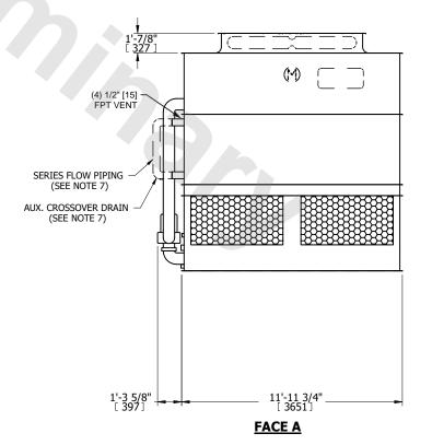
DRAWN BY: JLG NO. OF SHIPPING SECTIONS **SHIPPING** OPERATING HEAVIEST SECTION 16530 lbs+ [7500] kg+ 23080 lbs+ [10470] kg+ 14660 lbs+ [6650] kg+ WEIGHT WEIGHT WEIGHT
