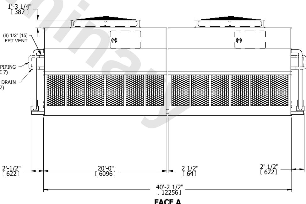
SHIPPING WEIGHT 54160 lbs+ [24570] kg+ OPERATING WEIGHT 83100 lbs+ [37695] kg+ HEAVIEST SECTION WEIGHT 22570 lbs+ [10240] kg+ NO. OF SHIPPING SECTIONS 4 DRAWN BY: JLG
