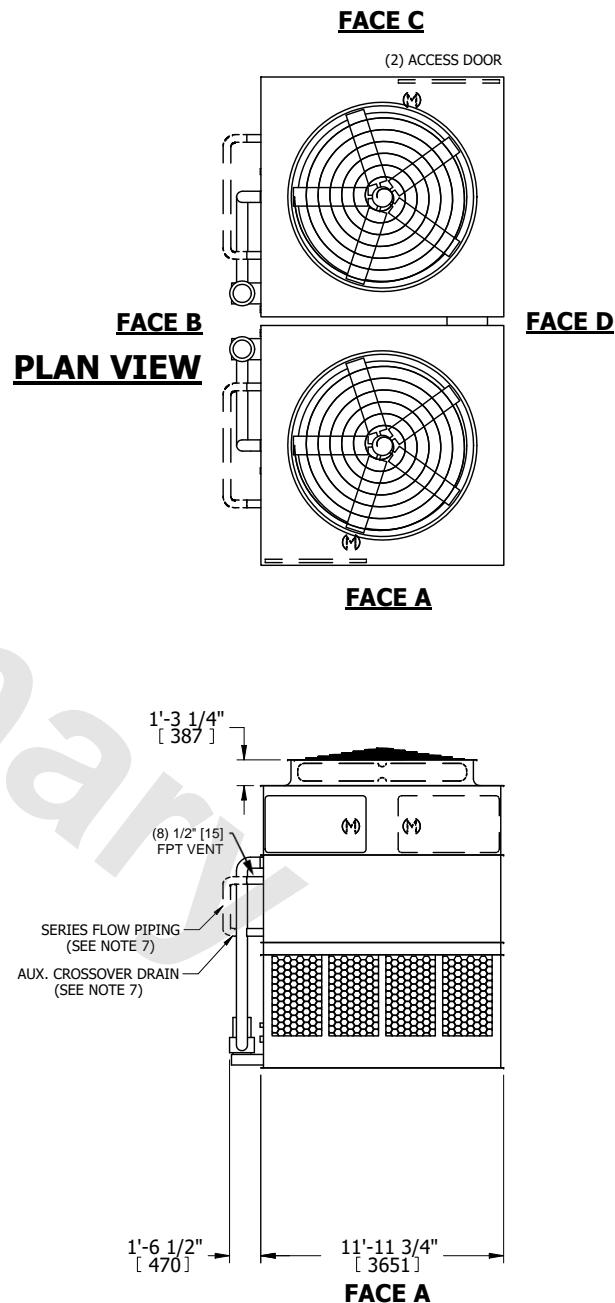
SHIPPING WEIGHT 40880 lbs+ [18545] kg+ OPERATING WEIGHT 59760 lbs+ [27110] kg+ HEAVIEST SECTION WEIGHT 17730 lbs+ [8045] kg+ NO. OF SHIPPING SECTIONS 4 DRAWN BY: JLG
