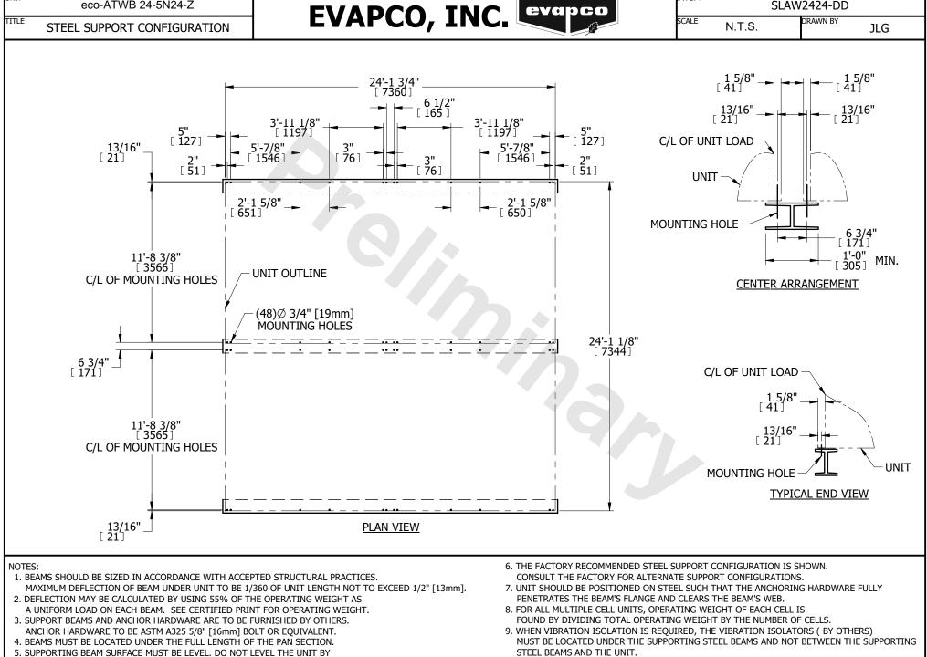
PLACING SHIMS BETWEEN THE UNIT MOUNTING FLANGE AND THE SUPPORTING BEAM.
