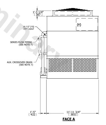
SHIPPING WEIGHT 22290 lbs+ [10115] kg+ OPERATING WEIGHT 31770 lbs+ [14415] kg+ HEAVIEST SECTION WEIGHT 19740 lbs+ [8955] kg+
