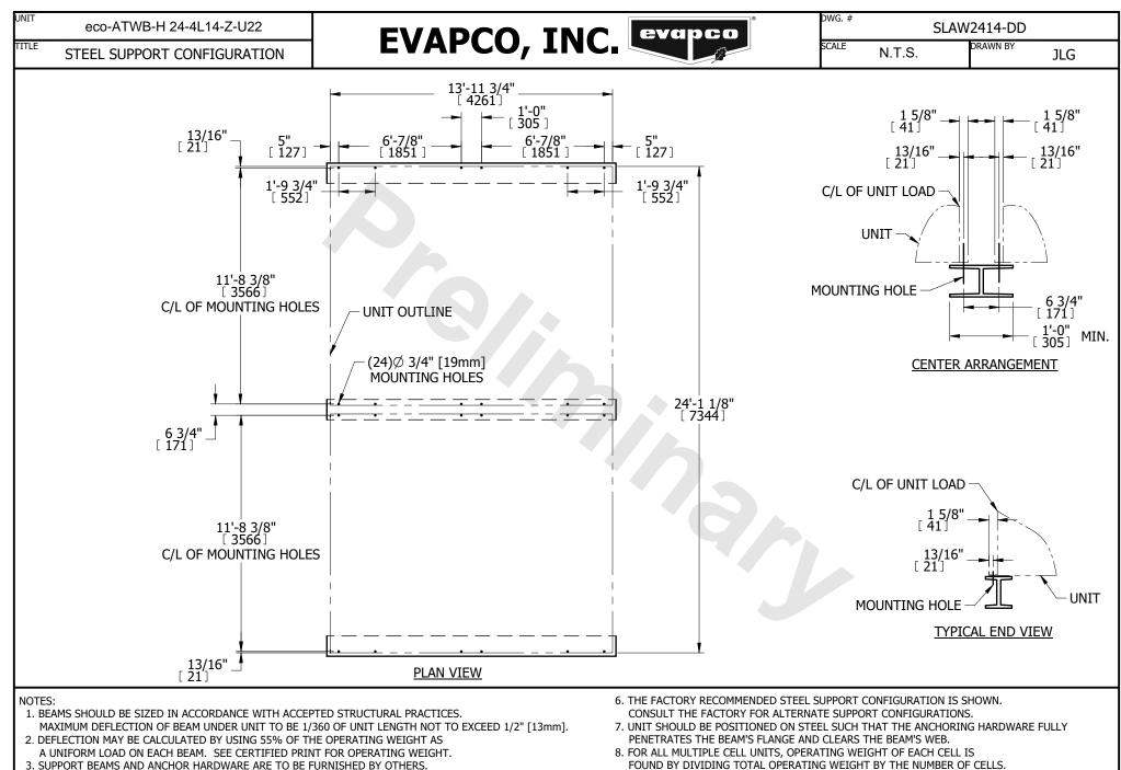
ANCHOR HARDWARE TO BE ASTM A325 5/8" [16mm] BOLT OR EQUIVALENT.
