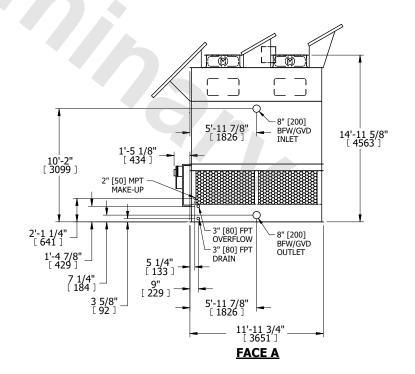
DRAWN BY: MBG NO. OF SHIPPING SECTIONS **SHIPPING** OPERATING HEAVIEST SECTION 10180 lbs+ [4620] kg+ 15880 lbs+ [7205] kg+ 3930 lbs+ [1785] kg+ WEIGHT WEIGHT WEIGHT
