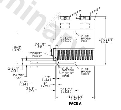
NO. OF SHIPPING SECTIONS **SHIPPING** OPERATING HEAVIEST SECTION 10180 lbs+ [4620] kg+ 15880 lbs+ [7205] kg+ 3930 lbs+ [1785] kg+ WEIGHT WEIGHT WEIGHT
