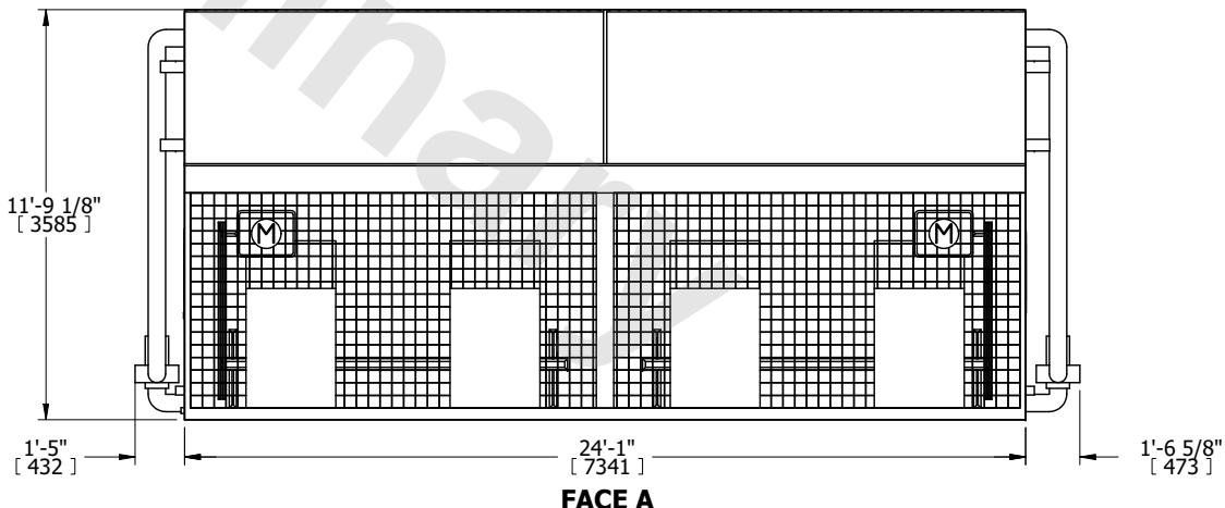
SHIPPING WEIGHT 21600 lbs+ [9800] kg+ OPERATING WEIGHT 34000 lbs+ [15425] kg+ HEAVIEST SECTION WEIGHT 7320 lbs+ [3325] kg+ NO. OF SHIPPING SECTIONS 3 DRAWN BY: TLS
